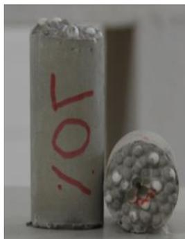
**Figura 4 – Amostra com 10% de EPS.
