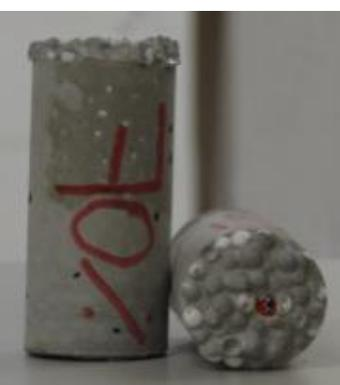
**Figura 10 – Amostra com 70% de EPS.
