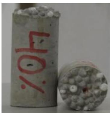
**Figura 7 – Amostra com 40% de EPS.
