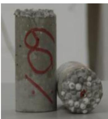
**Figura 9 – Amostra com 60% de EPS.
